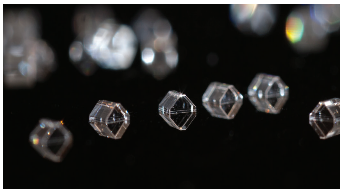
Single crystal CVD diamond prisms for use in spectroscopy applications.
