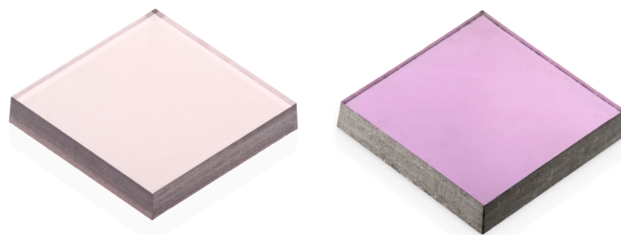
Figure 2: DNV B1 (left) and DNV B14 (right) CVD diamond samples
