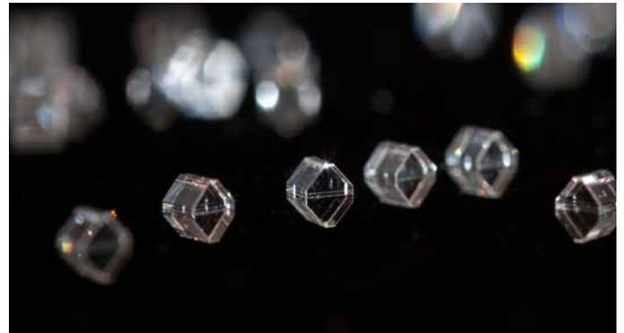
Single crystal CVD diamond prisms for use in spectroscopy applications.
