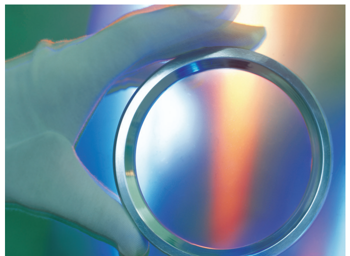
Microwave CVD diamond components have a transmission spectrum from 220 nm to >50 µm. They also conduct heat better than any other material.
